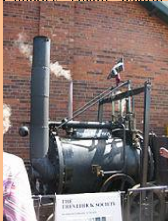
A replica of Richard Trevithick's 1801 road locomotive 'Puffing Devil'
