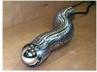
of the robot. You can think of a caterpillar moving by changing the shape of its body to match a sinusoidal wave. Similarly, snakebots can move by adapting their shape to different periodic functions.
